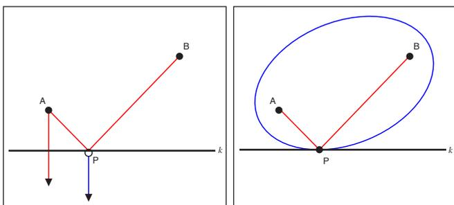
\* A string is tied to a pin at B, passes through a frictionless ring with a weight attached, and then over a pin at A; the weight is lifted by pulling on the string, until the ring touches line  $k$ .
